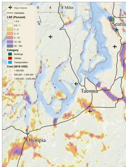
**Figure 1:** *Htot* (LSE) values for 2001 Nisqually event projected into NAD 1983 (2011) StatePlane Washington North FIPS 4601 (Meters). *Htot* values were calculated from this by the summation of each cell’s area multiplied with its LSE value:
