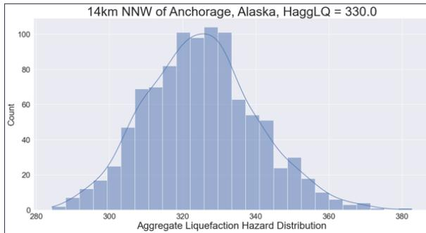
**Figure 3:** Histogram and probability distribution function of 1,000 draws from beta distribution of 2018 Anchorage event's aggregate liquefaction hazard.
