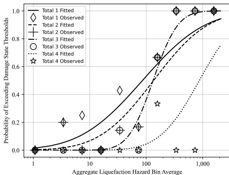
**Figure 2:** Probability of failure observations and resulting fragility functions using four liquefaction cost-based damage states found in table 1.
