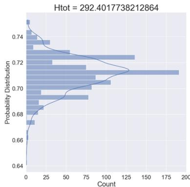
**Figure 5:** Histogram and distribution of resulting 1,000 fragility function probability values for DS 1 at  $H_{tot} = 292.40$  using 1,000 draws from each event's beta distribution.
