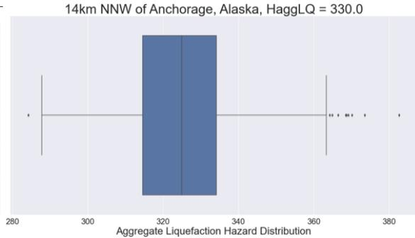
**Figure 4:** Box plot of 1,000 draws from beta distribution of 2018 Anchorage event's aggregate liquefaction hazard.
