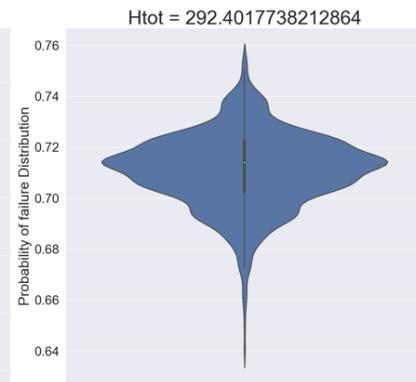
**Figure 7:** Violin plot of resulting 1,000 fragility function probability values for DS 1 at  $H_{tot} = 292.40$  using 1,000 draws from each event's beta distribution.
