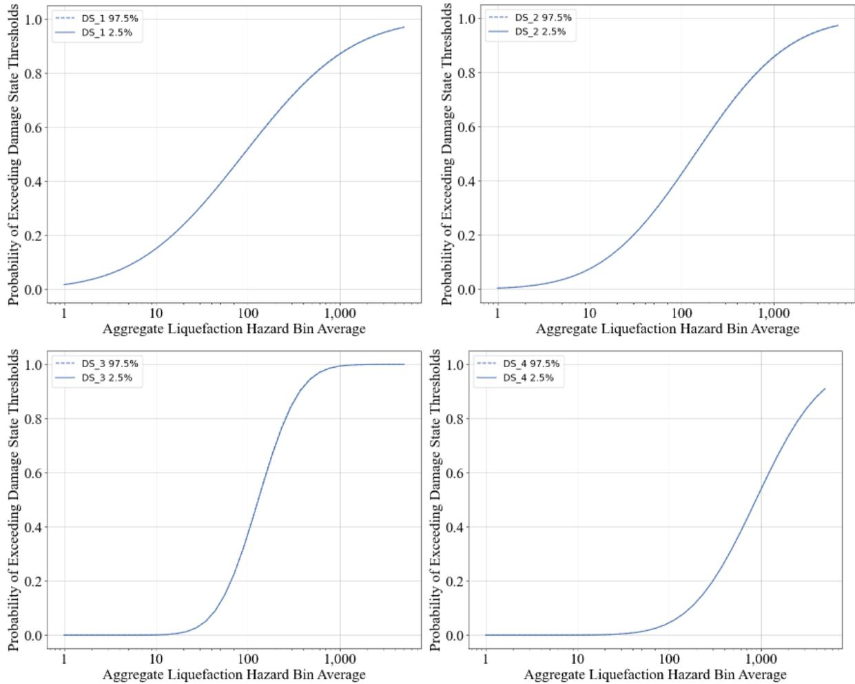
**Figure 9:** Confidence intervals of probability values along each fragility curve which have a 95% of containing the true probability population mean. The probability data did not have a very wide distribution at each excitation measure, resulting in a relatively narrow confidence interval.
