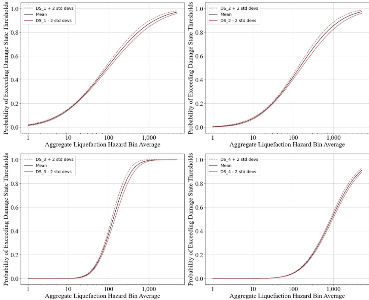
**Figure 8:** Mean and prediction intervals of  $\pm 2$  standard deviations from the mean of all 1,000 resulting values along the x-axis. 95% of observations fall within two standard deviations of the mean in a perfect normal distribution.
