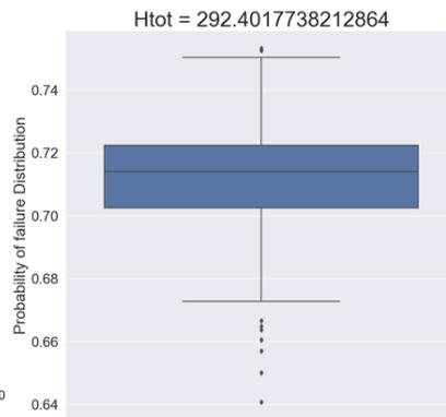
**Figure 6:** Box plot of resulting 1,000 fragility function probability values for DS 1 at  $H_{tot} = 292.40$  using 1,000 draws from each event's beta distribution.
